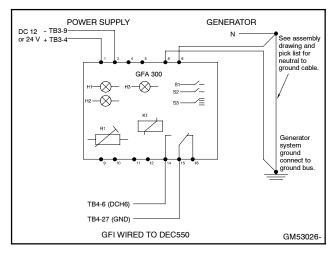
Figure 6-8 Ground Fault Connections
